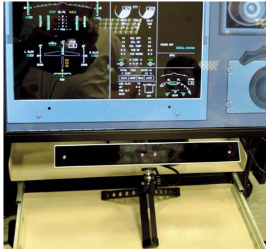
Figure 9. Eye tracker to register oculomotor activity
