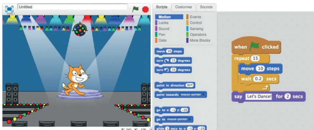
Fig. 3. The user interface of Scratch: we see similar connection between the program and its result in a rich visual environment
