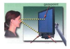
Video camera Eyegaze technology consists of a video camera and image processing software, which determines the eye's gazepoint on the screen
