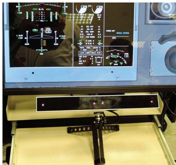
Fig. 3. Gazeport GP3 (Gazepoint Research Inc.) tracker, which was used for recording video oculography data
